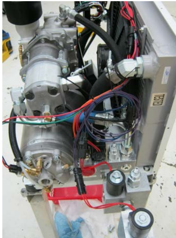
Figure 7 - Wires Connected and Bundled
