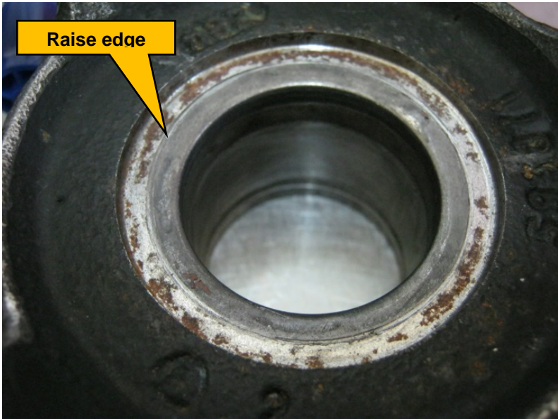
Figure 2.1 - Damaged Harmonic Balancer
