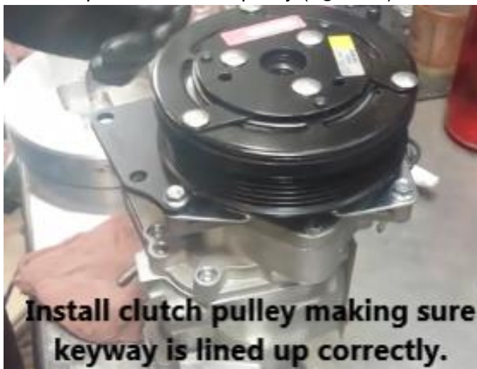
Figure 12 - Install clutch pulley
