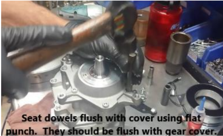
Figure 9 - Seat dowels
