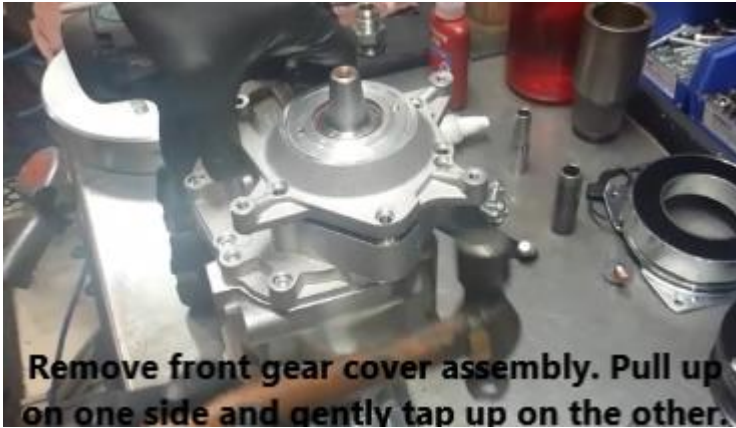
Figure 7 - Remove gear cover
