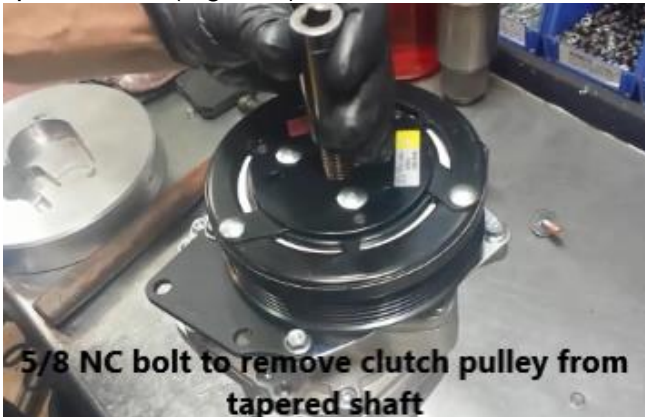
Figure 4 – Removing the clutch pulley
