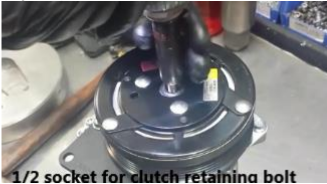
Figure 3 – Removing the clutch pulley
