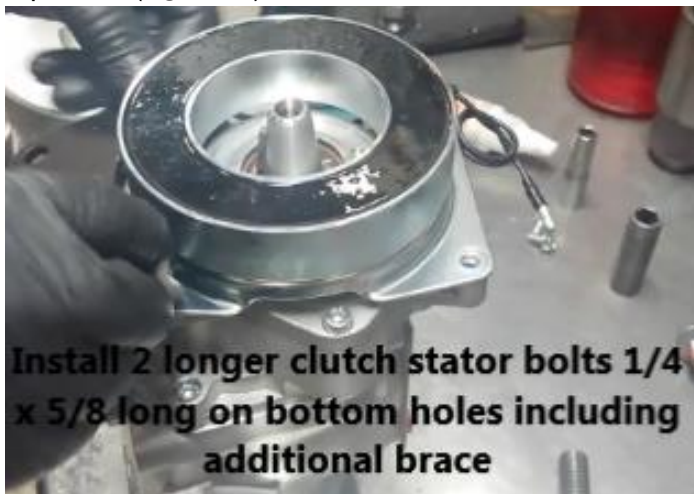
Figure 11 - Install clutch stator
