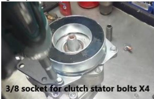
Figure 5 - Remove clutch stator
