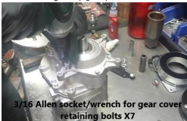
Figure 6 - Remove gear cover
