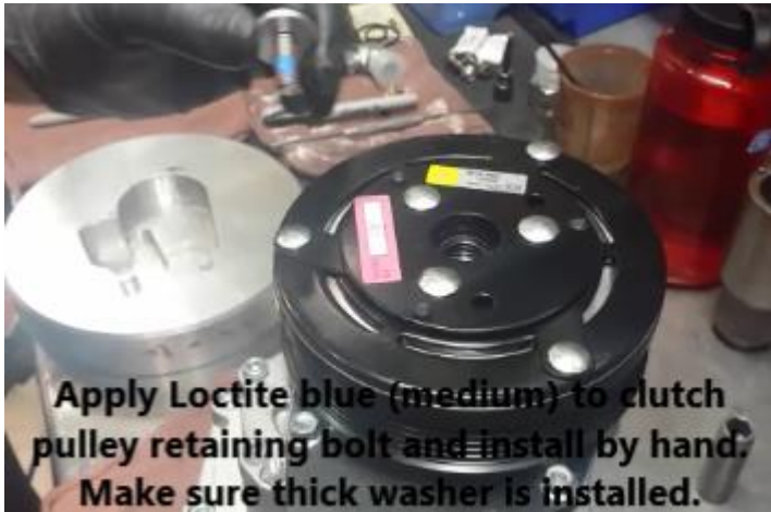
Figure 13 - Install clutch pulley
