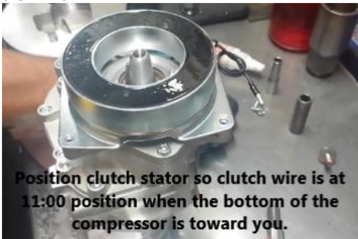
Figure 10 - Install clutch stator
